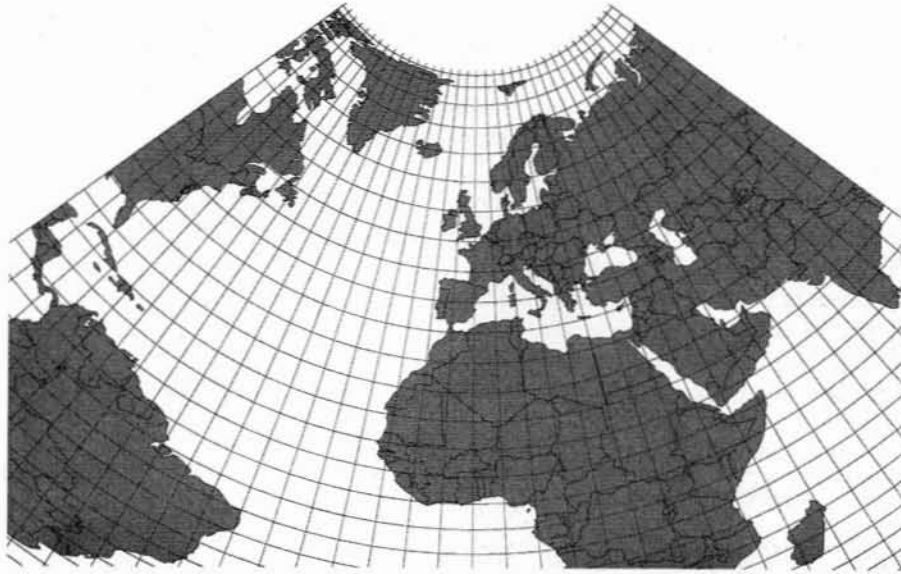
Figure 10.4 Albers equal area (conic) with standard parallels at 20° and 60° N.
