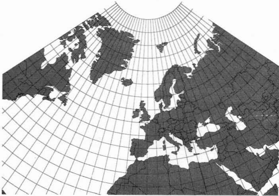
Figure 10.3 Conic equidistant projection with standard parallels at 20° and 60° N.
