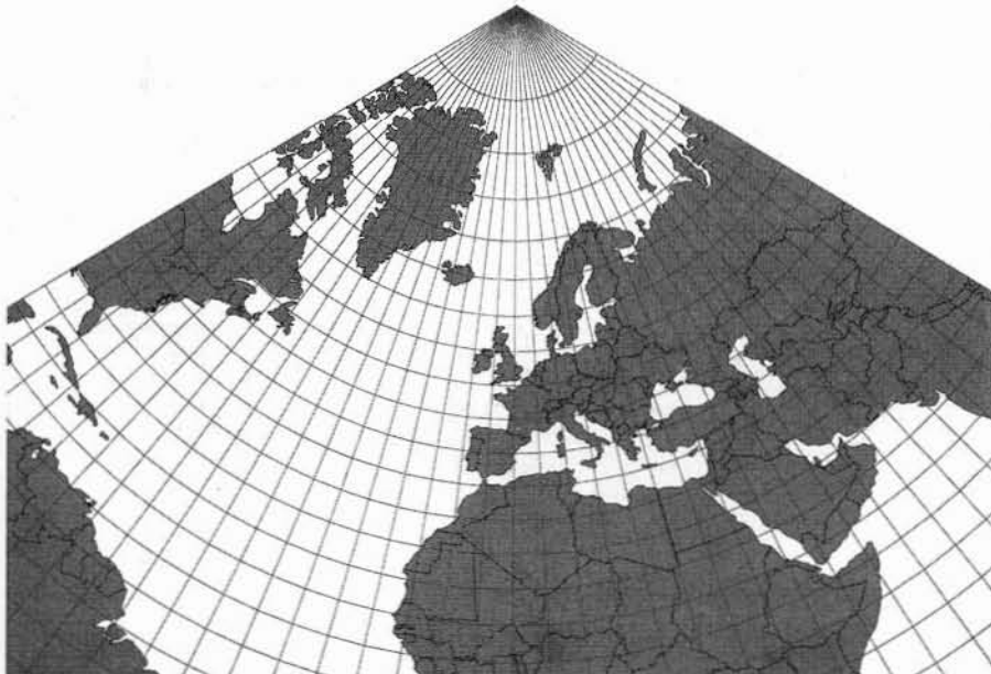
Figure 10.5 Lambert conformal conic projection with standard parallels at 20° and 60° N.
